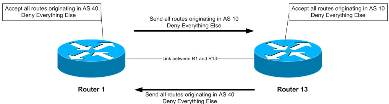
To verify that the regular expression works as intended, use the EXEC command “*show ip bgp regexp <regular-expression>*” to display all the paths that match the specified regular expression. Don’t forget that the command *clear ip bgp <neighbour address> [in|out]* is required to implement this filter.
